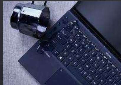
Keyboard Spill Resistance Test Liquid type: Water, coffee and coke Quantity : 66 cc, Duration : 3 mins
