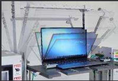
Hinge Test Subjects the laptop to up to 50,000 open-and-closed cycles
