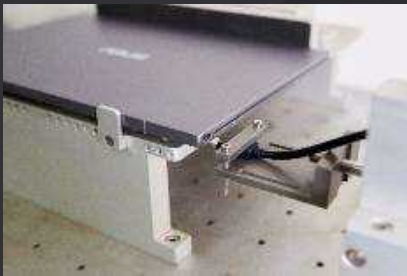
Port Durability Test 5,000 times tests to ensure the physical durability of I/O ports
