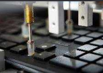
Keyboard Durability Test They're tested up to 10,000,000 keystroke lifespan
