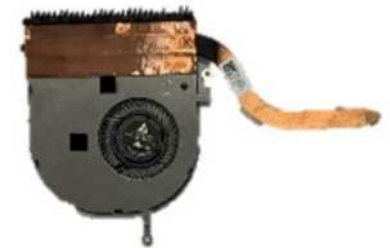
B9440's Fan structure
