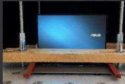
Shock Test Withstand 6 harsh shocks in each direction at the speed of 150G/2.5ms
